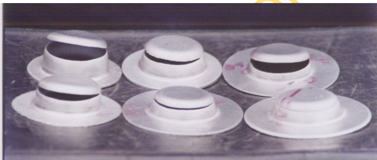
Fig. 1: Broken cups using 64, 65 and 70/33mm draw ratios
