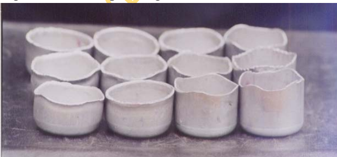
Fig. 2: Four sets of cups of varying thicknesses showing ears formed at the rims.
