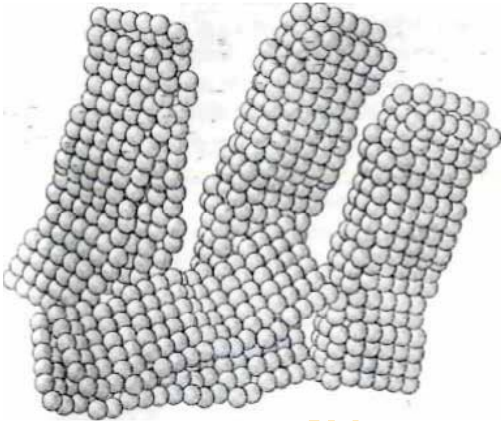
Figure 2.2 Microstructure of a Microporous Carbon
